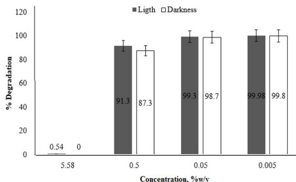
Figure 1. Photo-degradation of norbixin solutions in different concentrations, exposed to solar simulator at 1000 Wm<sup>-2</sup> for 6 hours
